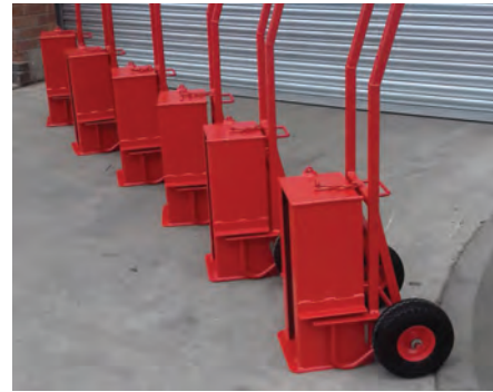
Used to hold various test weights for a single lift at a high SWL, primarily used for testing purposes
