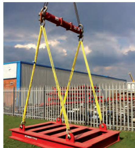
Used to hold various test weights for a single lift at a high SWL, primarily used for testing purposes
