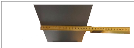
Fig. 42: Measuring flange width
