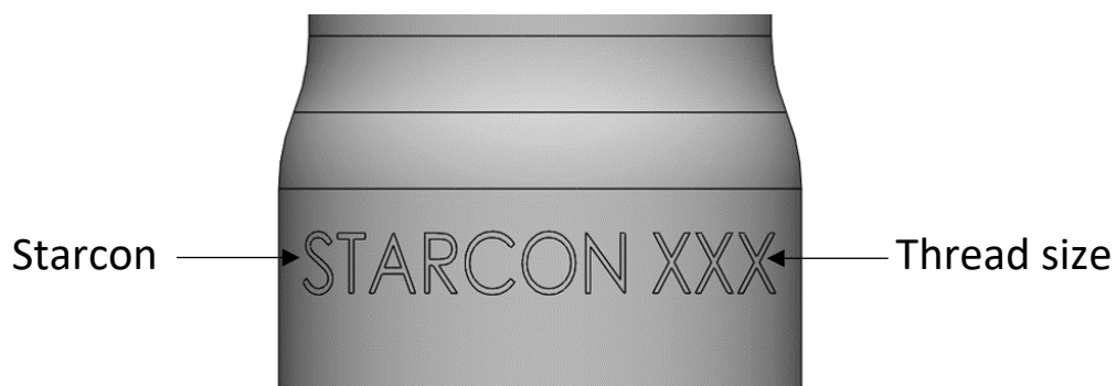
Figure 2 Marking on the cylinder of the insert for fastening.
