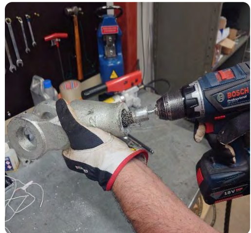
Removing dirt by using a wire brush
