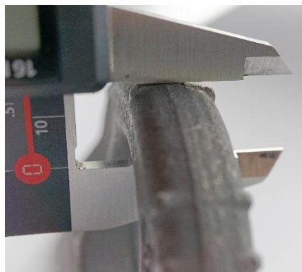
Maximal permissible wear: 5 % (see table 1)
