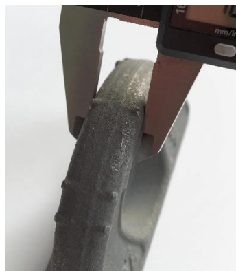
Maximal permissible wear: 5 % (see table 1)
