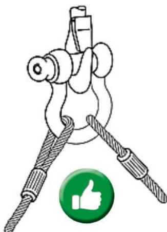
Fig. A.4 Correct - use two ropes with eyes
